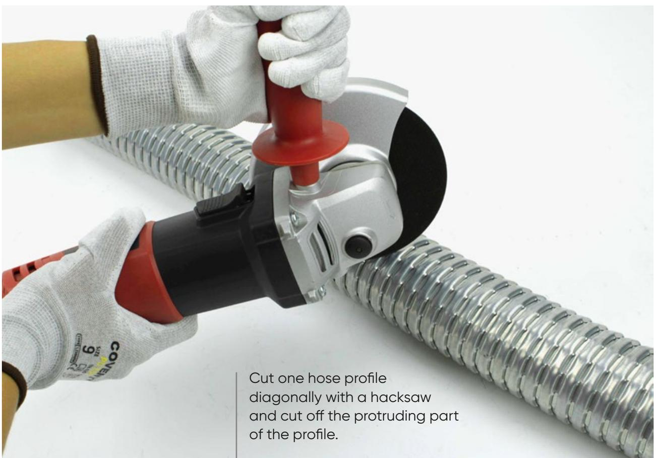
Cut one hose profile diagonally with a hacksaw and cut off the protruding part of the profile.
